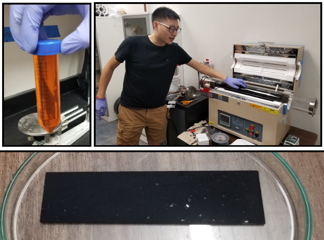
Figure 10. Above: Chemical Vapor Deposition Procedure: Toluene and Iron Catalyst (Left) and Tube Furnace (Right). Below: Resulting sample with deposited carbon nanotube layer.
