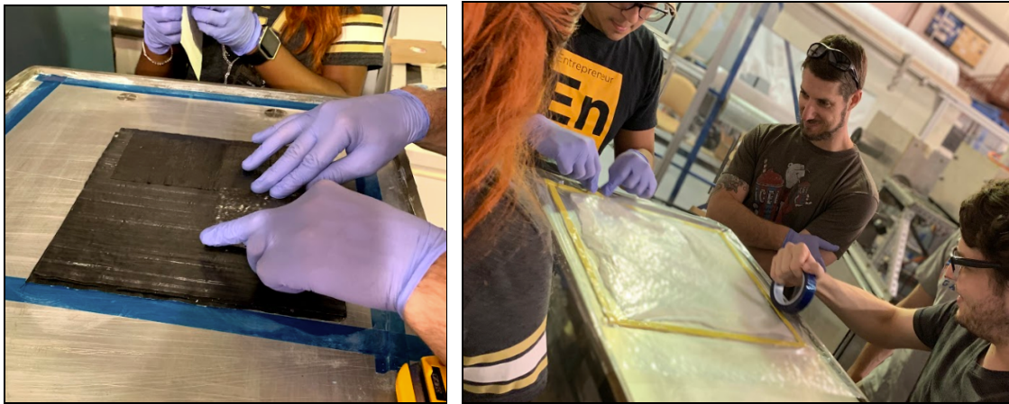
Figure 2. Laboratory procedures of layering pre-reg carbon fiber in an alternating pattern (LEFT) and sealing the product in preparation for vacuum and compression (RIGHT).
